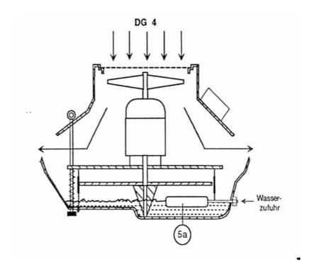
The waterlevel in the base tube is controlled by the lower flow switch of the two-step flow switch.
