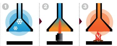
Put it into the fireplace. Open the chimney damper. Turn it on for 15-30 min. After 15-30 min switch it off and remove it. Put in firewood, strike a match and set fire.
