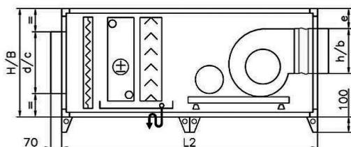
Note: All air-conditioning units with 6R heat exchanger are supplied with drop separator and condensate tray.
