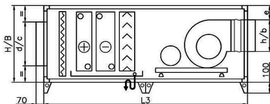
Note: All air-conditioning units with 6R heat exchanger are supplied with drop separator and condensate tray.
