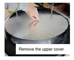
Once the upper cover is removed, all the internal components become accessible (see pictures below).
