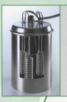
In the high-grade stainless steel cylinder, 1 to 5 high-quality, nickel-plated copper heating elements heat up the water according to the immersion boiler principle. The float switch and mechanical over temperature sensor work together allowing control of the water level and providing protection against dry-run.
