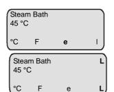
By pressing the key once, the **Essence Injector** Parameter is set continuously to off. This is indicated in the display by an e and results in no essence delivery into the steam bath.
