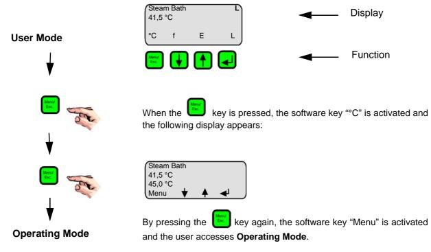
The sections below describe the configuration of the software menu, navigation through the menus, as well as display values, parameters and system functions.
