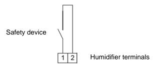
Safety interlock and Remote switch If both a circuit protection device and a remote switch are to be used, wiring is in series.
