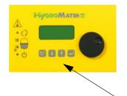
Keys are located below the display. Above each key, a context-based action (software key) is shown on the lowest line of the display (i.e. an "°C" key). The action is performed by pressing the key. The software keys in the display unit enable parameter modification.
