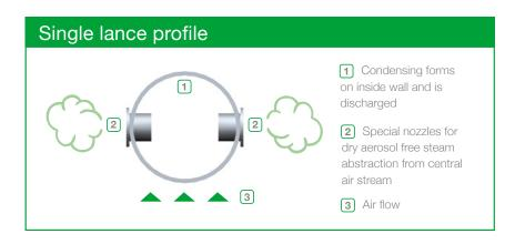
MultiLance systems are simple to install, maintenance-free and the high quality stainless steel components afford a long lifetime. Thanks to the special nozzle format the steam is obtained without aerosols from the middle of the lance, so that the downstream sensitive duct installations can be effectively protected from condensation.
