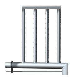
The HygroMatik MultiLance steam manifold systems are designed for use with extremely short absorption distances and are suitable for electrode and heater element steam humidifiers, as well as for steam injection systems. They can also be used with high flow velocities of up to 8 m/s in air ducts.
