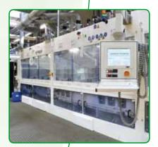
Additionally to the plus on controllability the Professional type offers all known advantages of our established HeaterLine units: a compact unit made of corrosion-resistant stainless steel with excellent access to its components.
