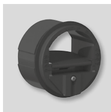
RDR Self-adjusting damper (150-250 Pa) that, fitted inside the duct, maintains constant airflow.
