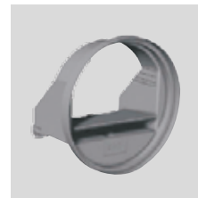
RD BP Specific low-pressure (20-100 Pa) and self-adjusting damper with sleeve to fit directly into the duct. 80mm diameter. Airflow: 15 or 30 m 3 /h.
