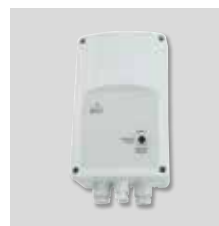
VAPZ Electronic single phase regulator that controls the fan speed with a simple contact (presence detector) or an analogical input, 0-10 V or 4-20 mA (from CO 2 probe or relative sensor).
