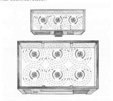
The choice the first unit's rotation is not important as long as the following units are installed with alternate rotations; it is not important what rotation the last unit has.
