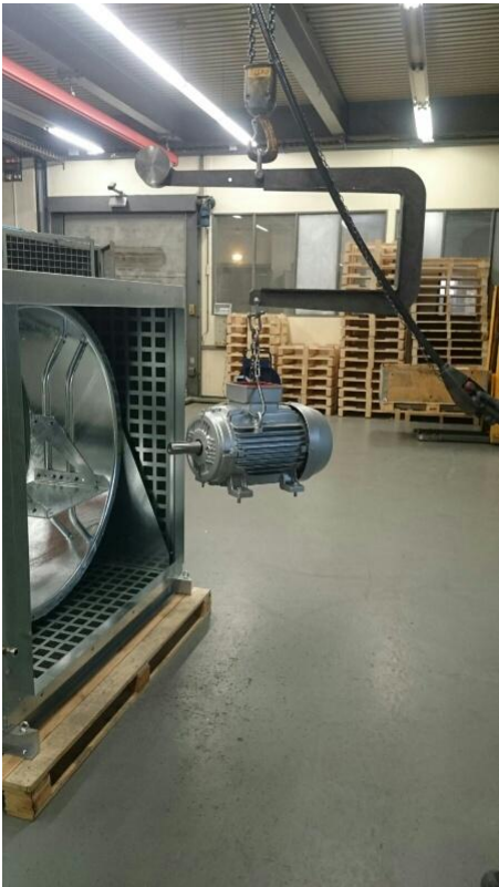
Fig 21 Typical motor lift for Long case axial
