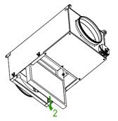
Remove used filters and replace them with the new ones, respecting the sense date of airflow found in the frame
