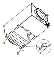
Rotate the lower stops with shape triangular (a) holding the prefilter.
