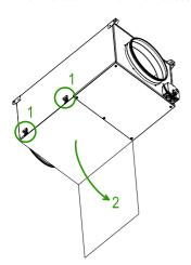
Remove the filter registration cover by turning the existing closing hands on the side and back loosened of these (1). Then, tilt the lid towards the side opposite the closing hands (2).
