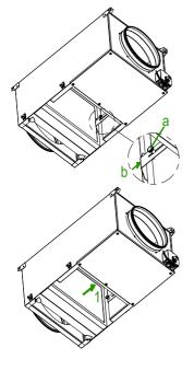
To release the filter or filters, loosen the two threaded knobs that hold each support (a), and move the arms until leaving enough space to remove the filter or filters (b).
