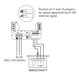
Using the control accessory AERO-REG CONTROL, it is possible to control the speed of the fans from an external sensor (CO2, humidity, pressure). See the details on connection in the AERO-REG CONTROL instructions.
