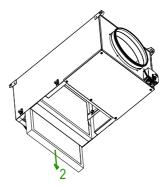
Release the prefilter, making it slide by the guides (2).
