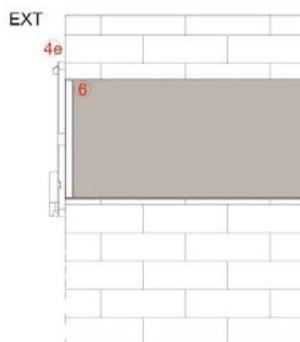
Insert the centring diameter of the wall attachment (4e) into the integrated tube (6).
