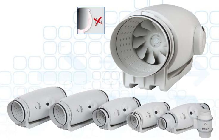
Low profile "Mixed-flow" fans with sound-absorbent fitted with rubber gaskets on the inlet and outlet to insulation, manufactured in plastic material with an external connection box, a body that can be dismantled and with speed controlable 230 V 50 Hz motor,
