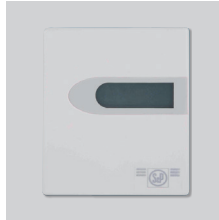
VRPZ Electronic control with display for single phase 230V-50/60Hz fans. Analogical input 0-10V or 4-20mA: The fan works proportionally to the input value with adjustments of the minimum and maximum values of the inputs and outputs.
