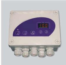
VRPZ Electronic control with display for single phase 230V-50/60Hz fans. Analogical input 0-10V or 4-20mA: The fan works proportionally to the input value with adjustments of the minimum and maximum values of the inputs and outputs.
